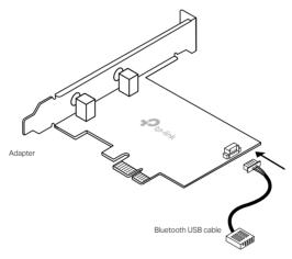
3. Locate an available PCIE slot and carefully insert the adapter.
